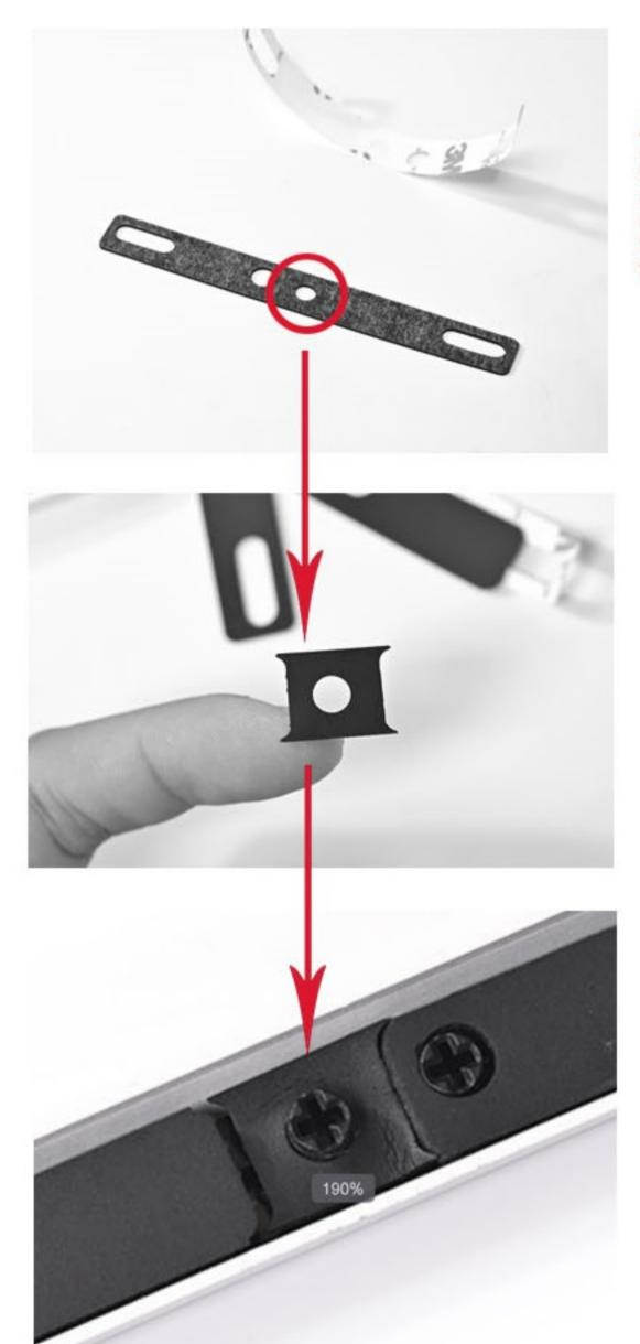
After installation of the two long pieces of foam, use the middle section of the thinner foam strip to surround the part of the spacebar stem that will have the switch stem inserted into it. A thinner piece of foam is used so that it does not impede the movement of the switch stem.
